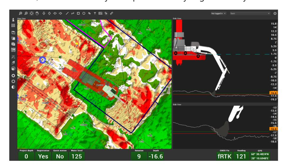
The dredge master can control the location of the dredger with regard to the depth map, as well as the location of the draghead against the bottom surface, target depth and boundaries. Moreover, an operator can always identify the areas where the works have not been performed yet.
